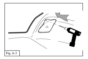
3. Repeat step 2 for other side of the vehicle using Right hand template.
